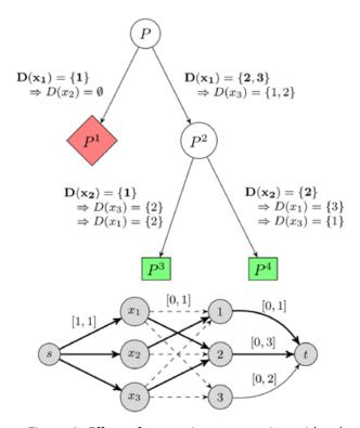
▲ Figure 2: Effect of constraint propagation with additional gcc constraint. The graph at the bottom illustrates the underlying maximum flow problem used for filtering the gcc constraint (see [6]). Thick edges correspond to the solution at subproblem *P* <sup>3</sup>, while dashed edges correspond to values that have been filtered out from the domains.
